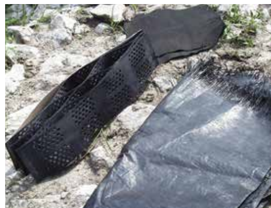
Polyethylene webbing may be used to stabilize crushed rock on hills, streambanks, and in streams. Photo by Shawn Shouse.
